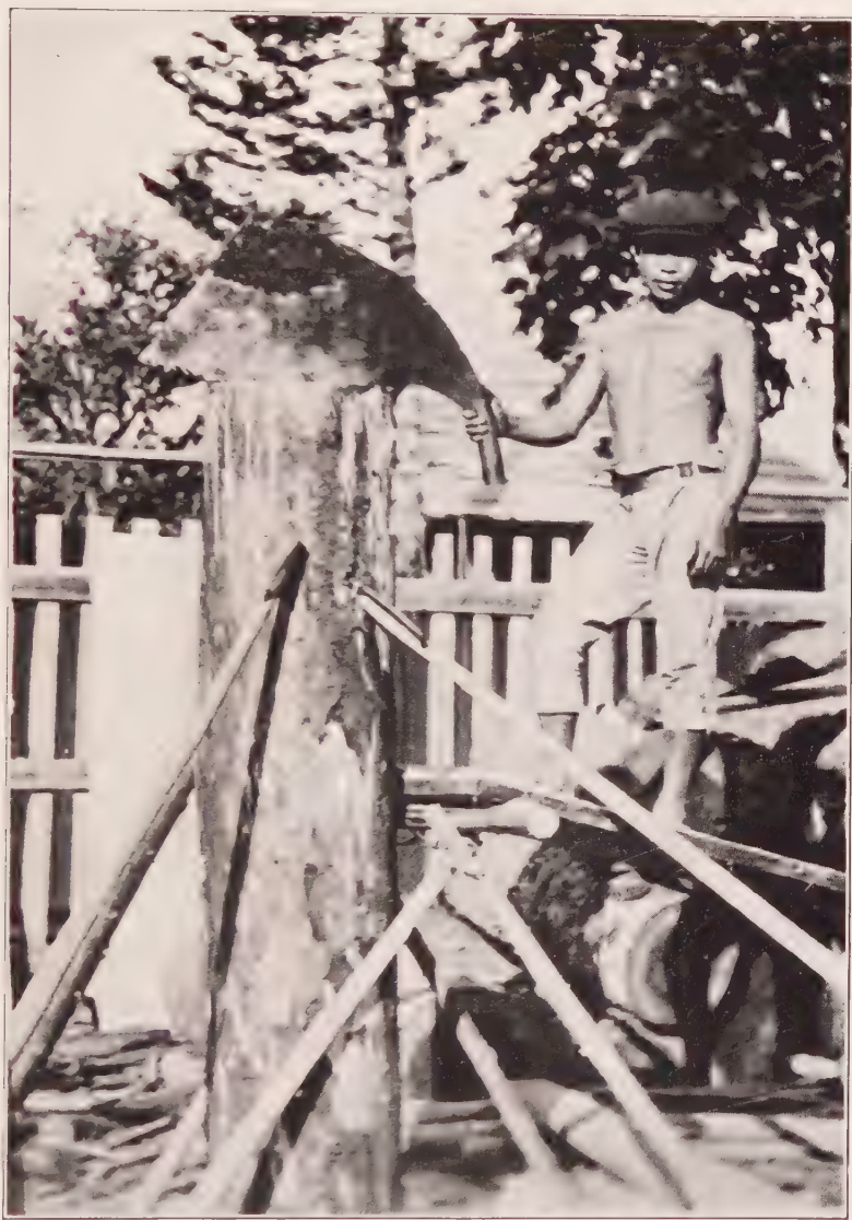
The saw the Japanese use for cutting logs into boards is a wide, short instrument like a butcher's cleaver with teeth filed in the blade.
